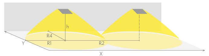
R1 distance from wall (X axis) R2 installation distance between lights (X axis) R4 distance from wall (Y axis) TWT1151WK
