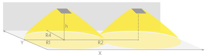
R1 distance from wall (X axis) R2 installation distance between lights (X axis) R4 distance from wall (Y axis) TWT4351WKH
