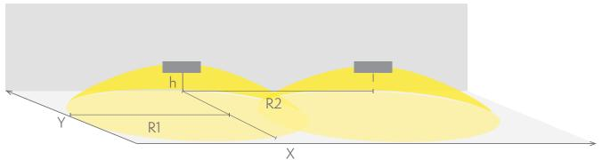
R1 distance from wall (X axis) R2 installation distance between lights (X axis) TWT1651WK
