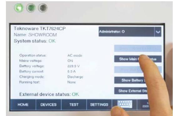
**Green LED lit:** Mains present, central battery unit in mains mode (AC)
